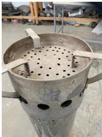
Fig. 1 Rig system (Rice Husk Stove)
