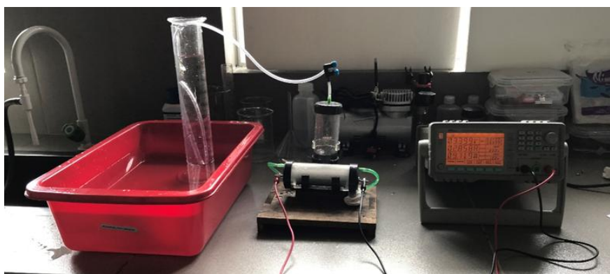
Fig. 5: Testing of the HHO Generator Unit with Bubbler Unit
