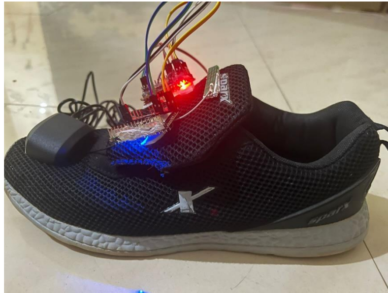
Fig.5.GPS Tracking System Setup
